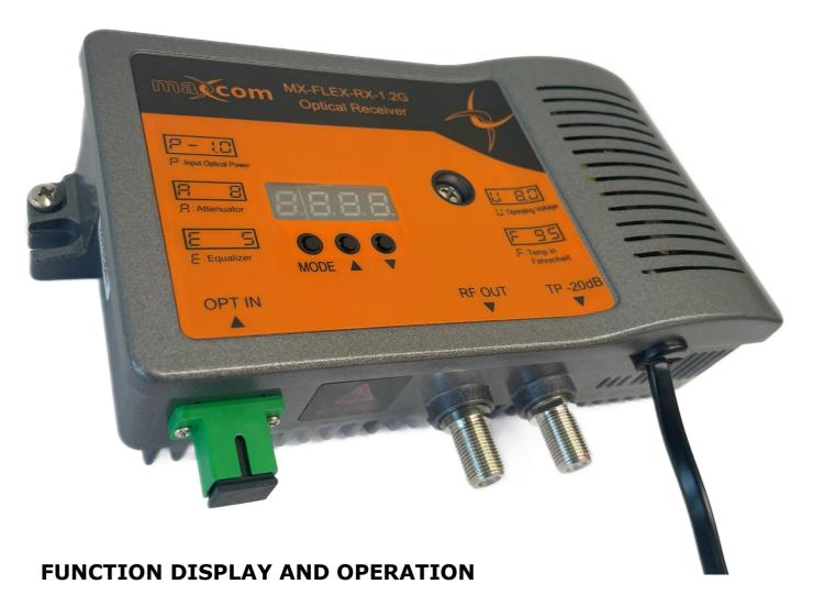
MODE: The Mode selection button steps through five different operating modes, press the MODE button for the corresponding status display. Note: LED screen will go into sleep after 1 minute.  $\blacktriangle$   $\blacktriangledown$  The Up/Down Arrow buttons allow the user to adjust the value.
